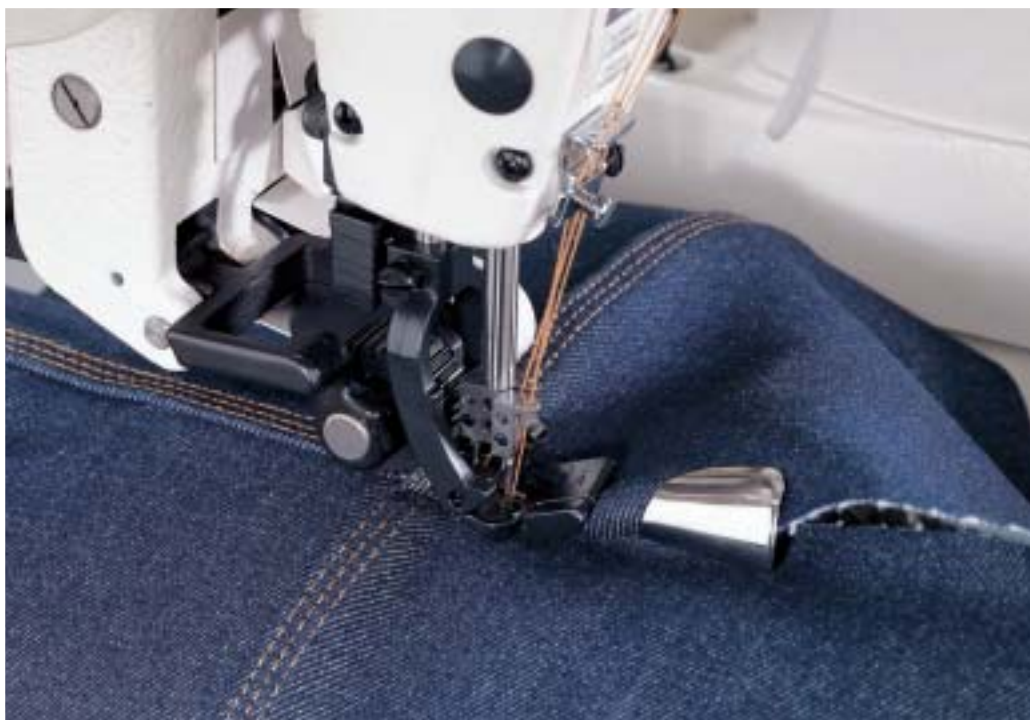
● Beautifully-finished seams are produced by smoothly feeding the overlapped parts of heavy-weight material.
