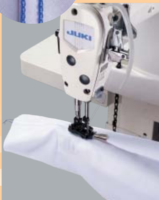
● Low-tension sewing ensures balloon stitches with a soft feeling.
